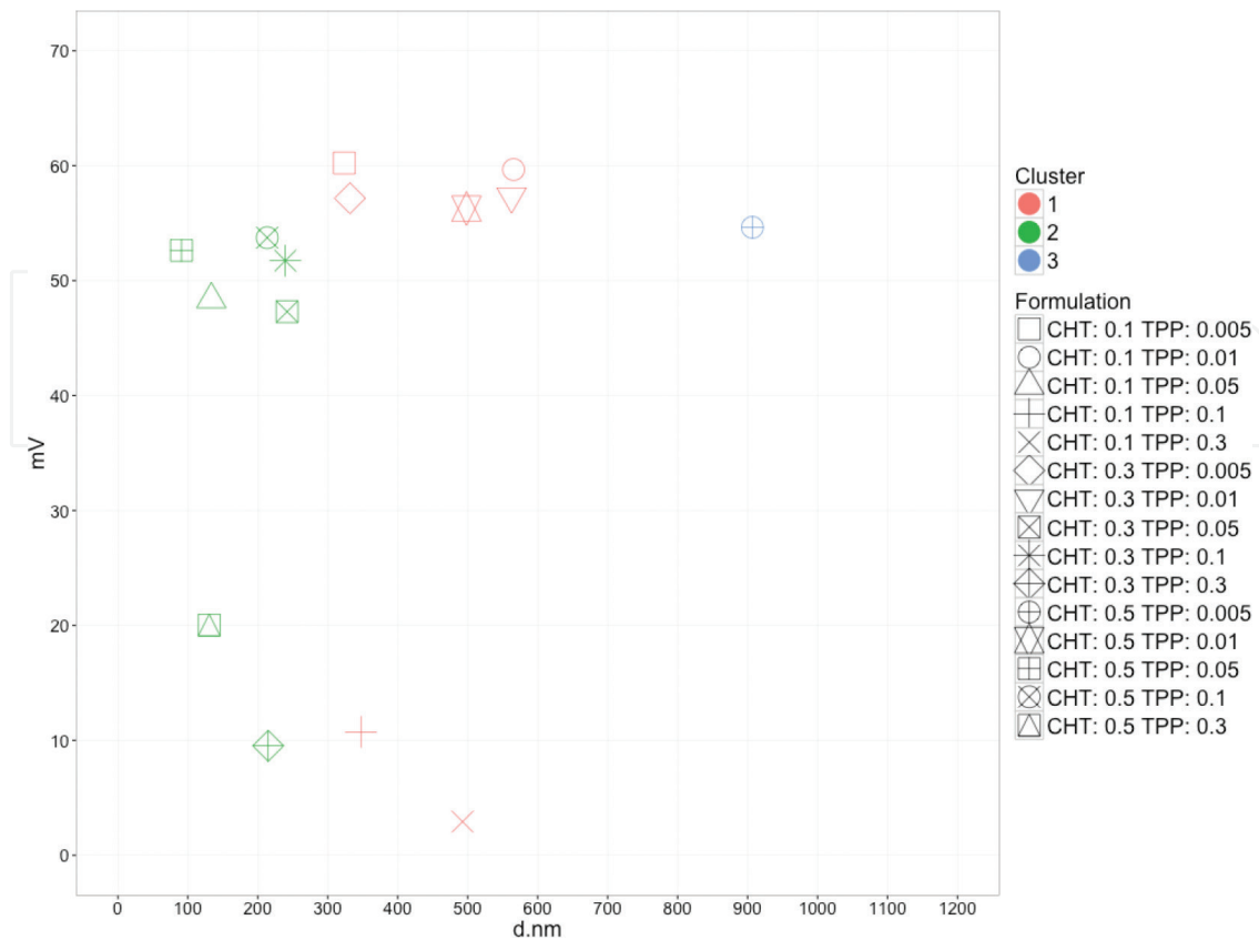
Figure 2. Scatter plot for diameter and surface charge of different CHT-NPs. The classification (clusters) was computed using the Hartigan-Wong k -means clustering algorithm [23]. Formulations indicate both CHT and TPP concentrations used for each nanoparticle type. The top left points in the green cluster (above 45 mV and below 300 nm) are the best delivery targets with respect to size and \zeta potential, which appear at medium to low concentrations of TPP (0.05–0.1% w/v) and mostly at medium and high concentrations of CHT (except for C with 0.1% w/v). Most experimentally found diameters are below 600 nm. In the case of surface charge, data are partitioned in two groups: above 40 mV and below 20 mV with no nanoparticle in the middle.
