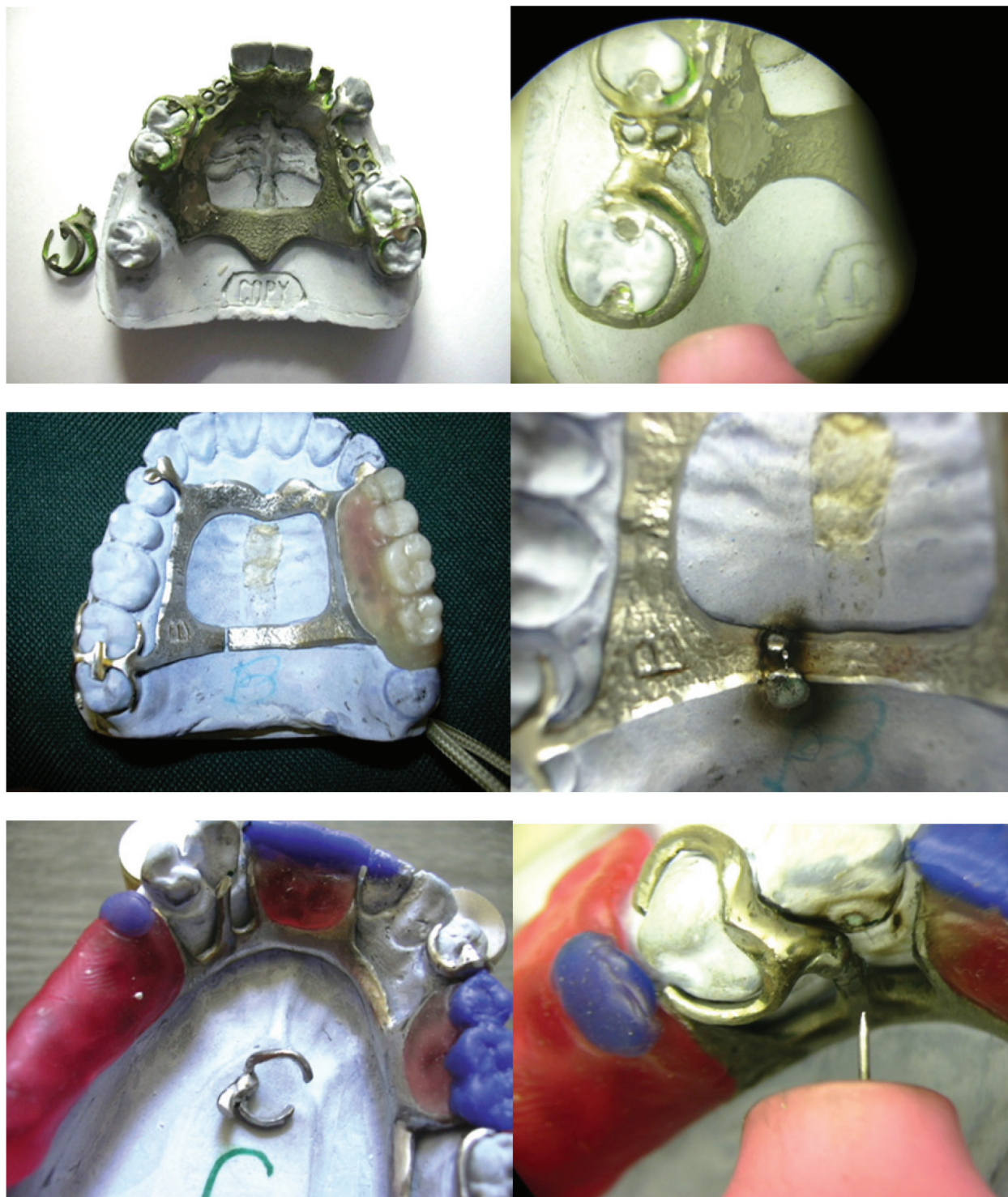
Figure 16. Some fractured metallic frameworks of removable partial dentures, before and after welding.
