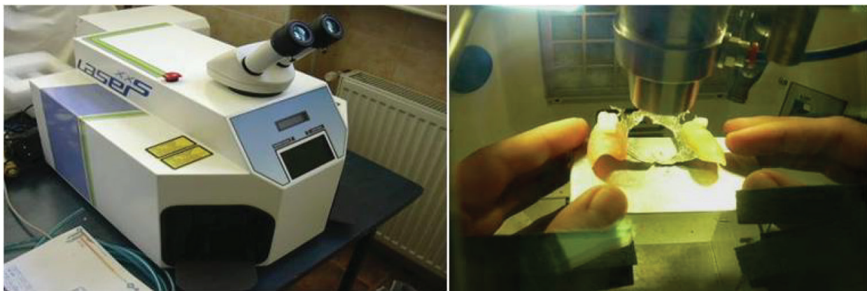
Figure 4. XXS laser welder for dentistry (Orotig) and its enlargement system.
