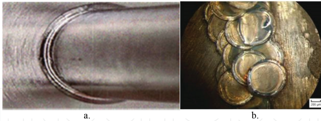
Figure 6. (a) Image of the welding cord. (b) Microscopic image of the welding points.
