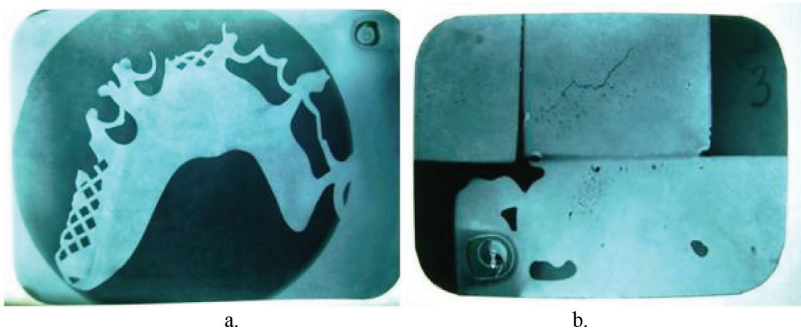
Figure 21. Radiographic images: (a) Metallic framework. (b) Welded plates.
