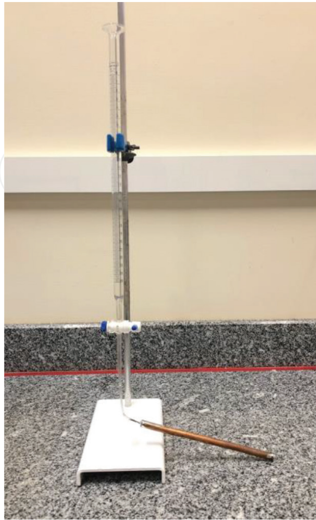
Figure 8. Filling station with the heat pipe.
