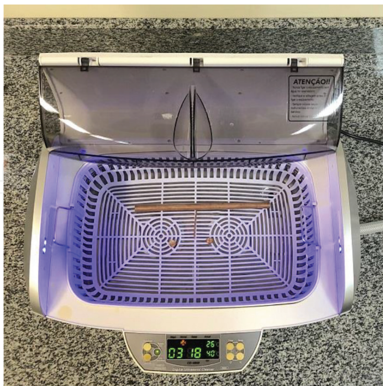
Figure 4. Cleaning procedure in the ultrasonic bath.
