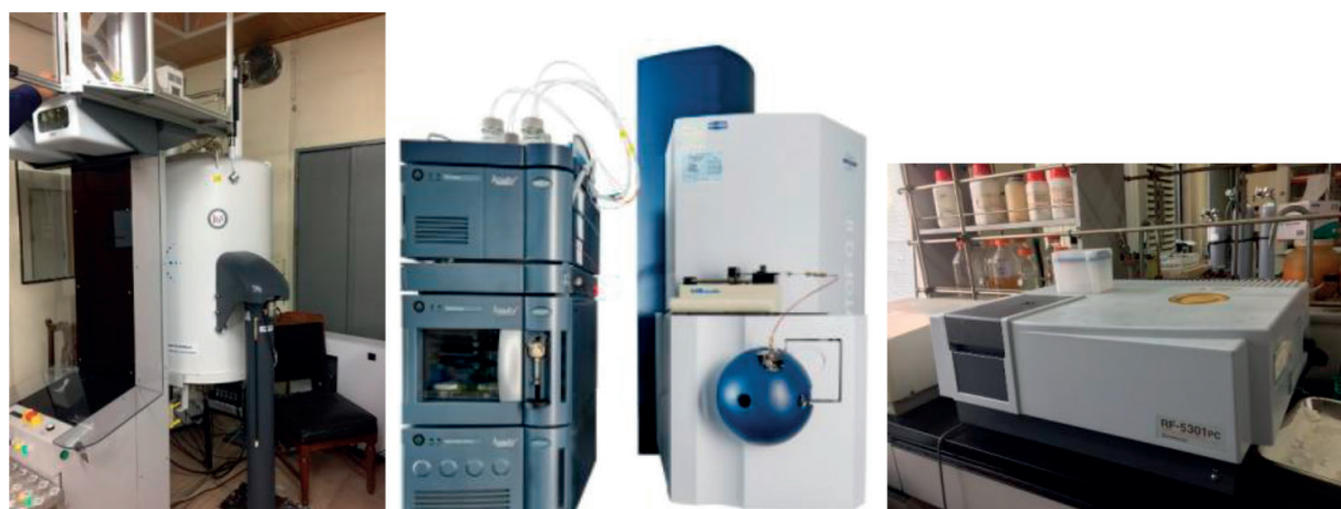
Figure 2. Instruments used in the scientific laboratory such as the multinuclear NMR spectrometer (left), high-resolution mass spectrometer (middle), and fluorimeter (right). (Photos acquired at KAIST (Daejeon, Korea); high-resolution mass spectrometer photo taken from kara.kaist.ac.kr ).
