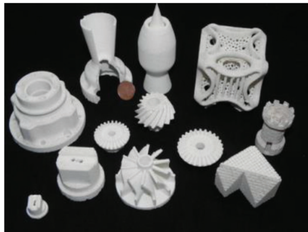
Figure 7. Pure alumina parts processed by SLM. Reprinted from [28], with permission of Cambridge University Press.
