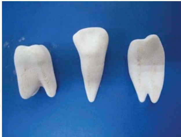
Figure 13. Teeth made by SLS under the optimized technical parameters Reprinted from [59], with permission of Emerald Publishing Limited.
