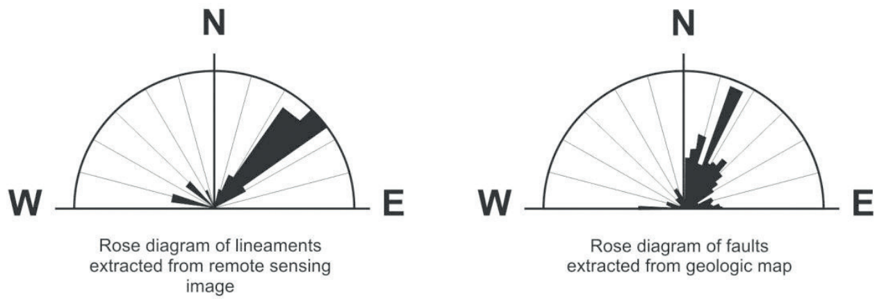
Figure 7. Rose diagrams extracted from geological map and shaded maps of the study area.
