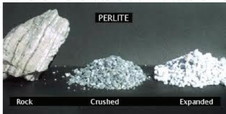
Figure 3. Morphology of perlite in its rock, crushed and expanded form.
