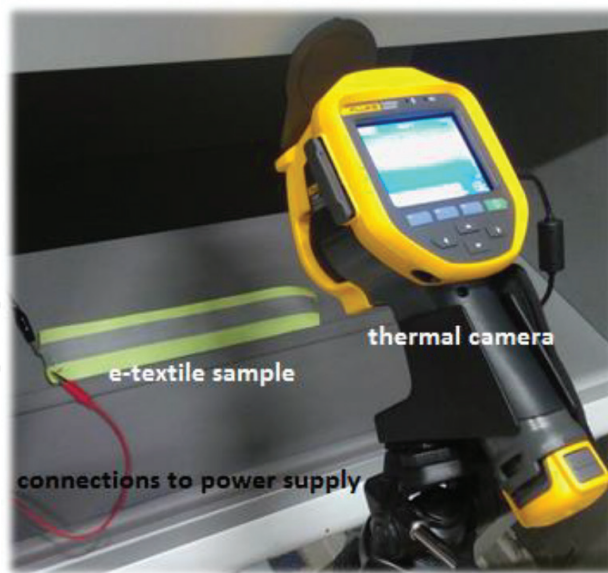
Figure 10. Testing set up to measure surface temperature.
