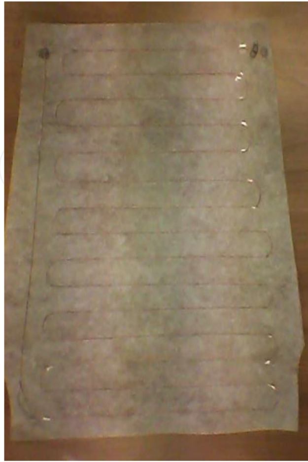
Figure 12. Placement of conductive yarn over interlining.
