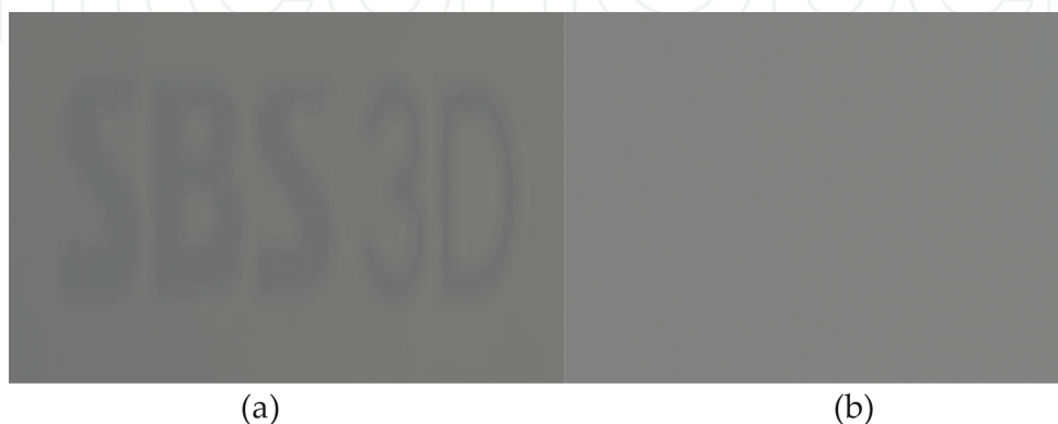
Figure 16. Image sticking test results (a) Before compensation, (b) After compensation.
