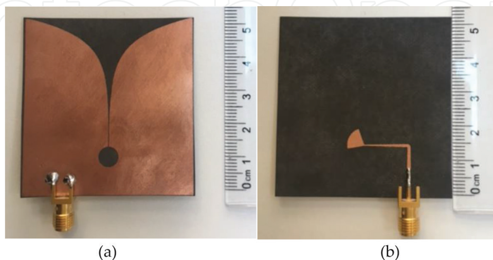
Figure 3. Fabricated Vivaldi antenna (a) top view; (b) back view.
