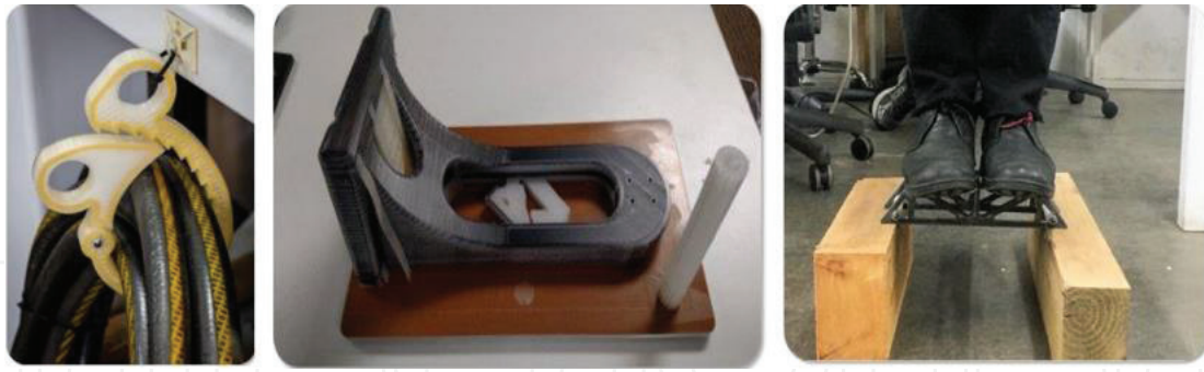
Figure 13. Holder with Kevlar reinforcement (left), head support for go-cart cars with carbon reinforcement (middle), and a structural part made of nylon and carbon fiber (right) [28].
