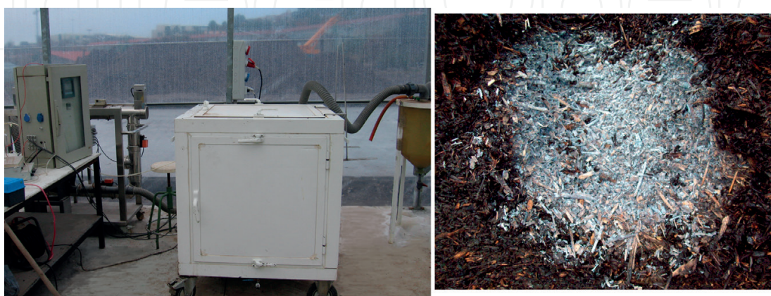
Figure 7. Composting reactor of 600 L equipped with a fan, recorder, and control of process parameters and biofilter (left) and colonized mixture of bulking agent with sewage sludge in 2:1 proportion in volume after process time (right).
