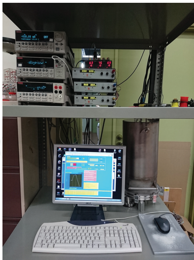
Figure 4. High temperature Seebeck measurement system: The electronics in the top shelf, the vacuum chamber (with the sample inside) in the back, and the computer with the control-software.
