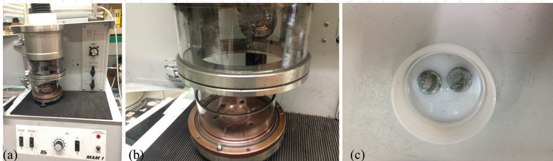
Figure 1. (a) Images of the mini arc furnace and (b) its water-cooled copper crucible, for synthesis of SnSe alloys materials. Pellets of powders of starting material are molten and then quenched in this crucible. (c) Typical disks of as-grown and then pressed intermetallic alloys.
