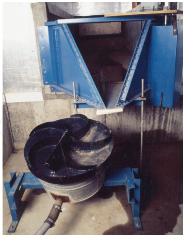
Figure 4. H flume and original Coshocton wheel rotating-slot sampler.
