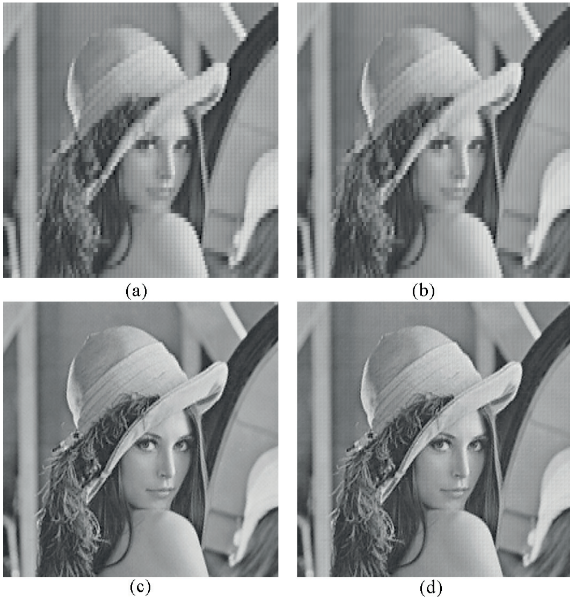
Figure 15. Compression with 2 and 8 original and periodic principal components. (a) Compression with two components (b) Compression with two components_{per} . (c) Compression with eight components. (d) Compression with eight components_{per} .
