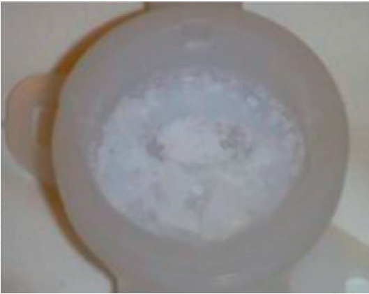
Figure 8. The clogged silica abrasive in slurry delivery loop.
