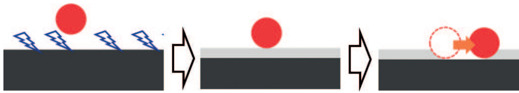
Figure 2. The schematic mechanism of material removal by CMP.
