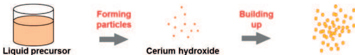
Figure 13. Synthesis of nano-sized cerium hydroxide abrasive (reprinted from Ref. [33] with permission from authors).
