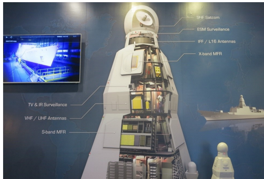
Figure 4 - SMk2, a high-end RADAR developed by Thales [3].
