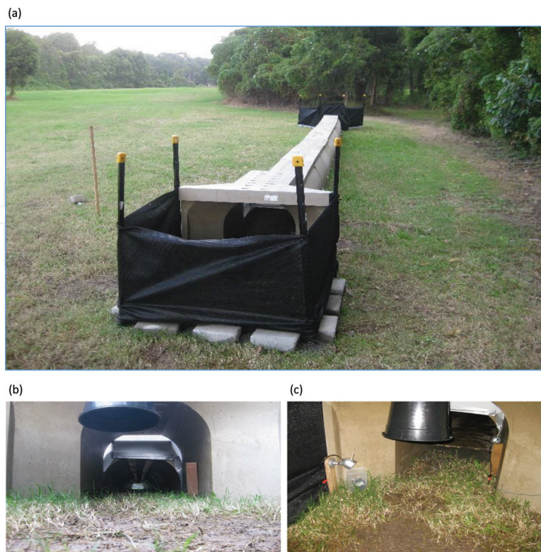
Figure 2. Experimental setup to study the tunnel-crossing behavior of amphibians. Experimental tunnel (ACO climate tunnel model KT 500) used to record amphibian-crossing movements, Photographs by Andrew Hamer (from ([52])). (a) Global view of the tunnel; (b) a view through the tunnel from the entrance arena; (c) view of the tunnel entrance with the infrared camera on the left and the temperature data logger next to the camera. The black plastic bucket is the raised acclimation chamber used for tested animals.
