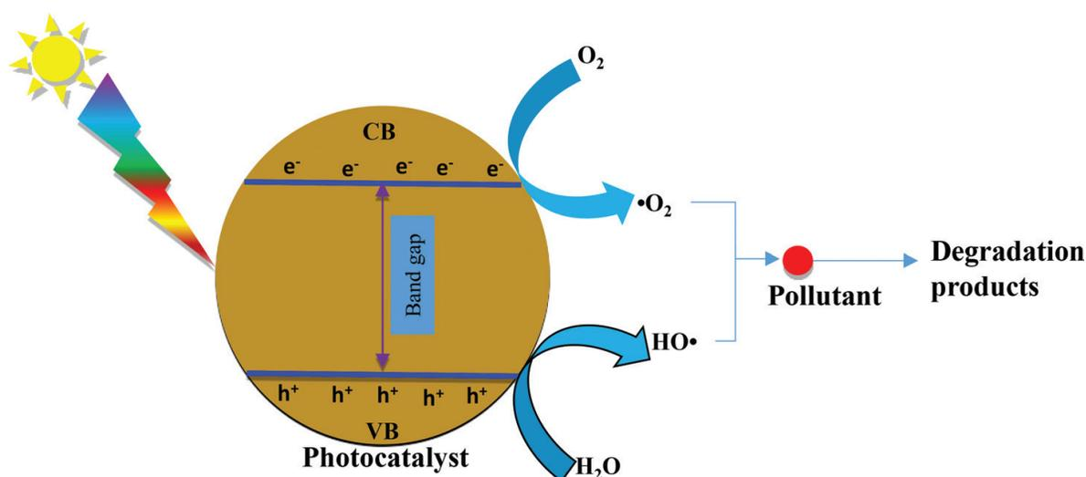
**Figure 3.** Mechanism of photocatalytic degradation of organic polluting.
