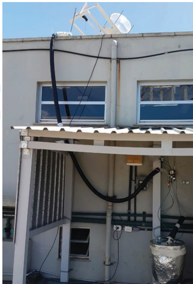
Figure 8. Prototype: non-transparent photobioreactor with internal illumination by plastic optical fibers, coupled to solar tracking.
