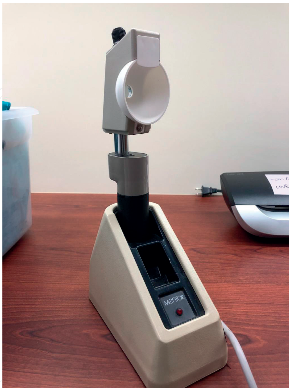
Figure 2. Brightness acuity test (BAT) commonly utilized as a glare source for glare testing. Elliot et al. [28].
