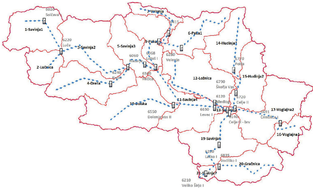
Figure 5. Modelling scheme of the Savinja River catchment with discharge gauging stations that were applied in this study.
