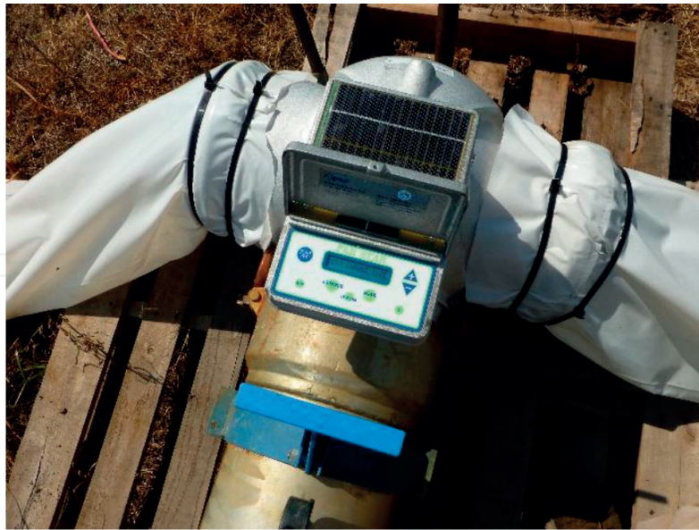
Figure 3. Surge valve used to improve distribution of furrow irrigation in fields.
