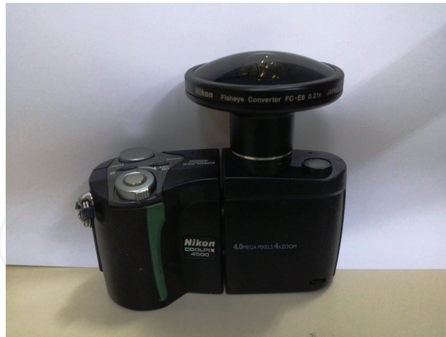
Figure 3. Camera and Nikon FC-E8 fisheye converter.
