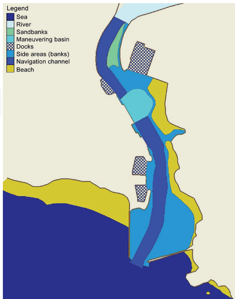
Figure 6. Materials (different roughness) considered in the analysis, in the section between the road bridge and immediately downstream of the bar.
