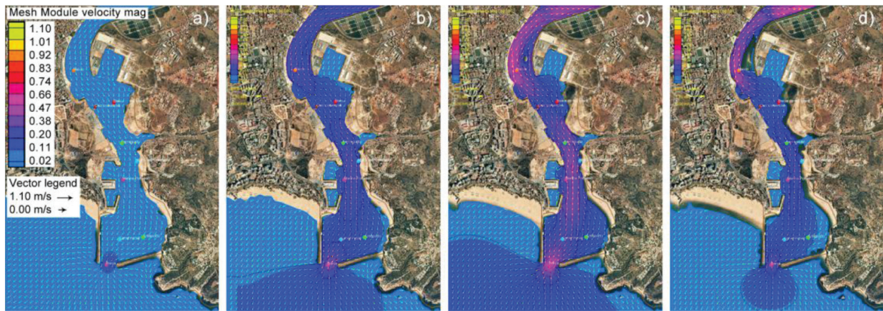
Figure 9. Reference situation. Results obtained during ebb flow: (a) 50, (b) 51, (c) 53 and (d) 55 hours.
