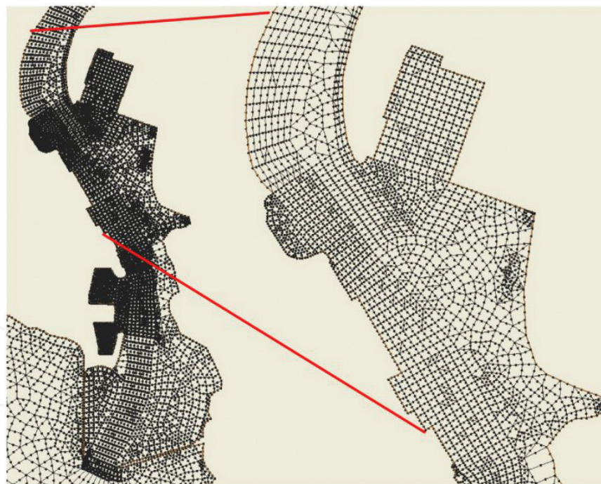
Figure 3. Details of the mesh in the estuary of the Arade River: the estuary and the zone that comprises the Dock of San Francisco, the fishing port, the commercial wharf and the Navy Pier and the maneuvering basin.
