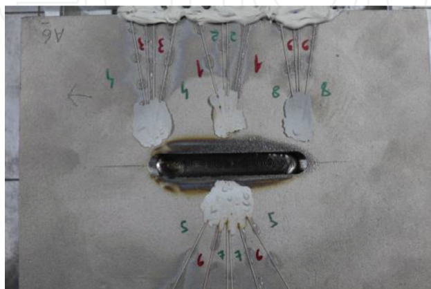
Figure 14. Specimen geometry and location of the thermocouples close to the slot.
