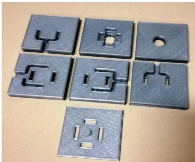
Figure 4. Printed layers of an ortho-mode transducer (OMT) based on turnstile junction, working in W-band.
