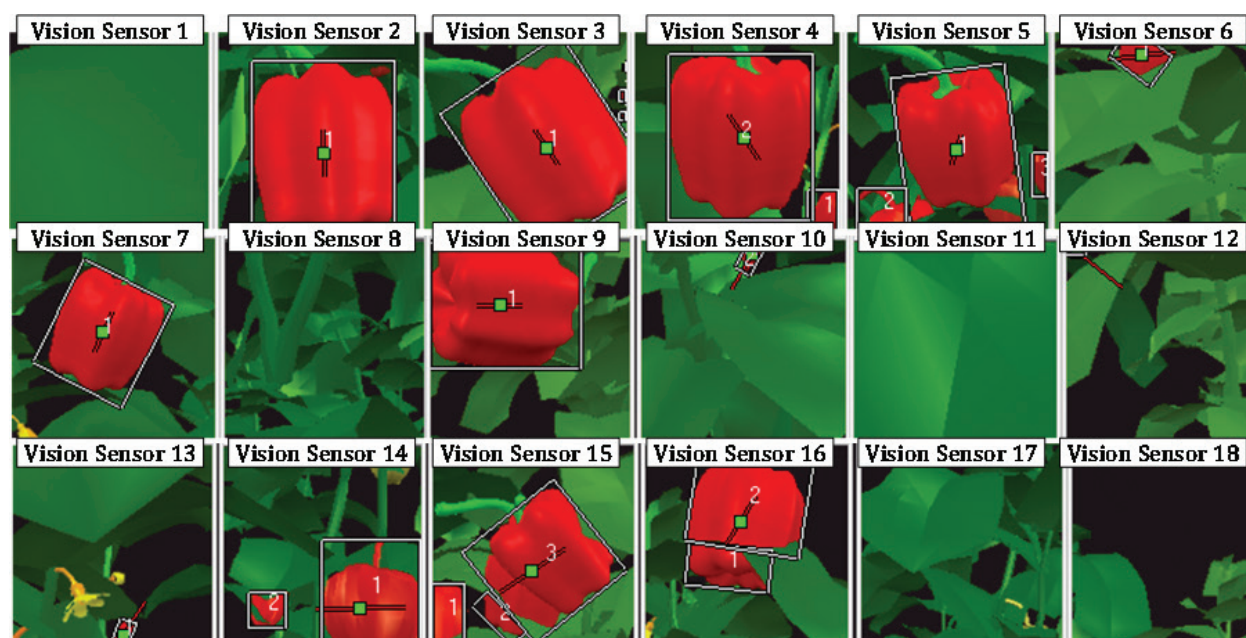
Figure 24. Simulation of robotic harvesting with arrays of linear actuators.
