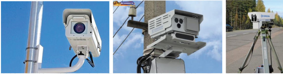
Figure 1. CCTV cameras and photoradar vehicle detector complexes.
