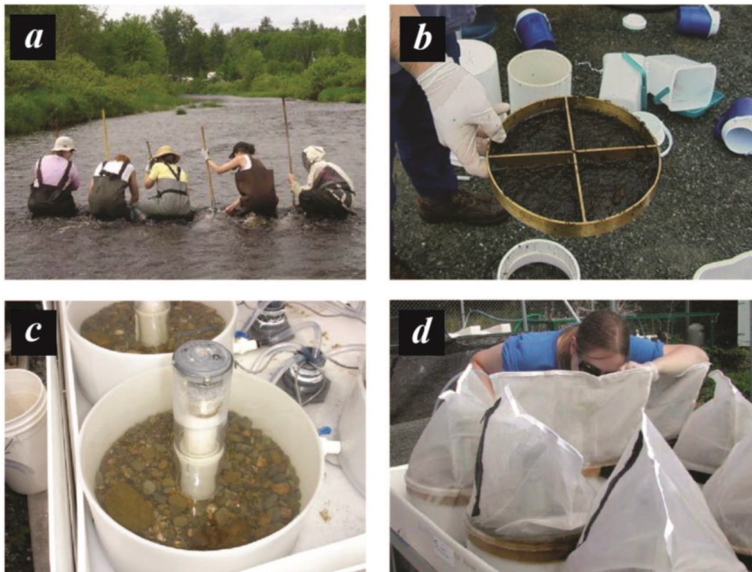
Figure 1. Outdoor, flow-through, stream mesocosms. (a) Benthic macroinvertebrates are collected by five samplers collecting 4 U-nets each. (b) The benthic community is then subsampled (four-way pie-plate subsampler shown). Community subsamples are then inoculated into replicate streams (e.g., ¼ of community sampled per replicate). (c) Each replicate stream is circular (0.065 m 2 and 10-L volume) and was also inoculated with five cobblestones and coarse and fine gravel. (d) After inoculation with benthic macroinvertebrates each stream is covered with 45 μm mesh to facilitate the daily collection of emergent insects.
