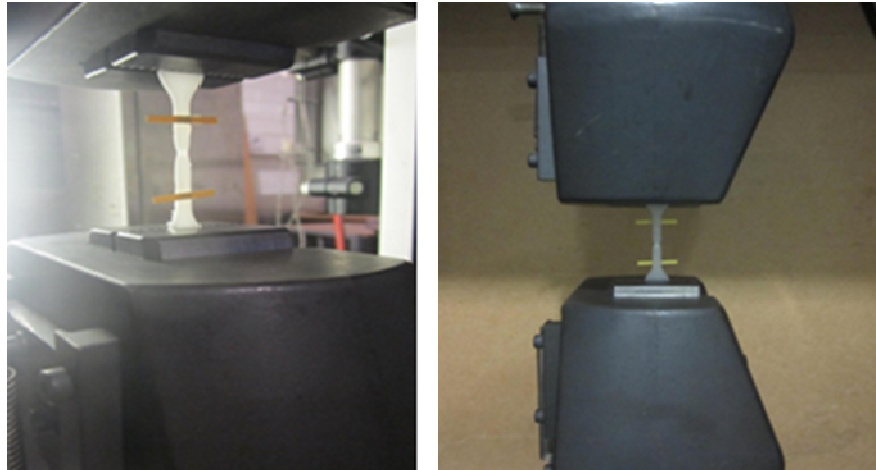
Figure 3.2: Tensile specimen edges gripped between tensile machine hands
