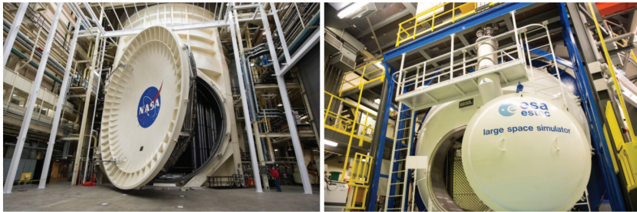
Figure 2. (Left) Chamber A – NASA Johnson Space Center’s and (Right) large space simulator (LSS) ESTEC test Centre, ESA.
