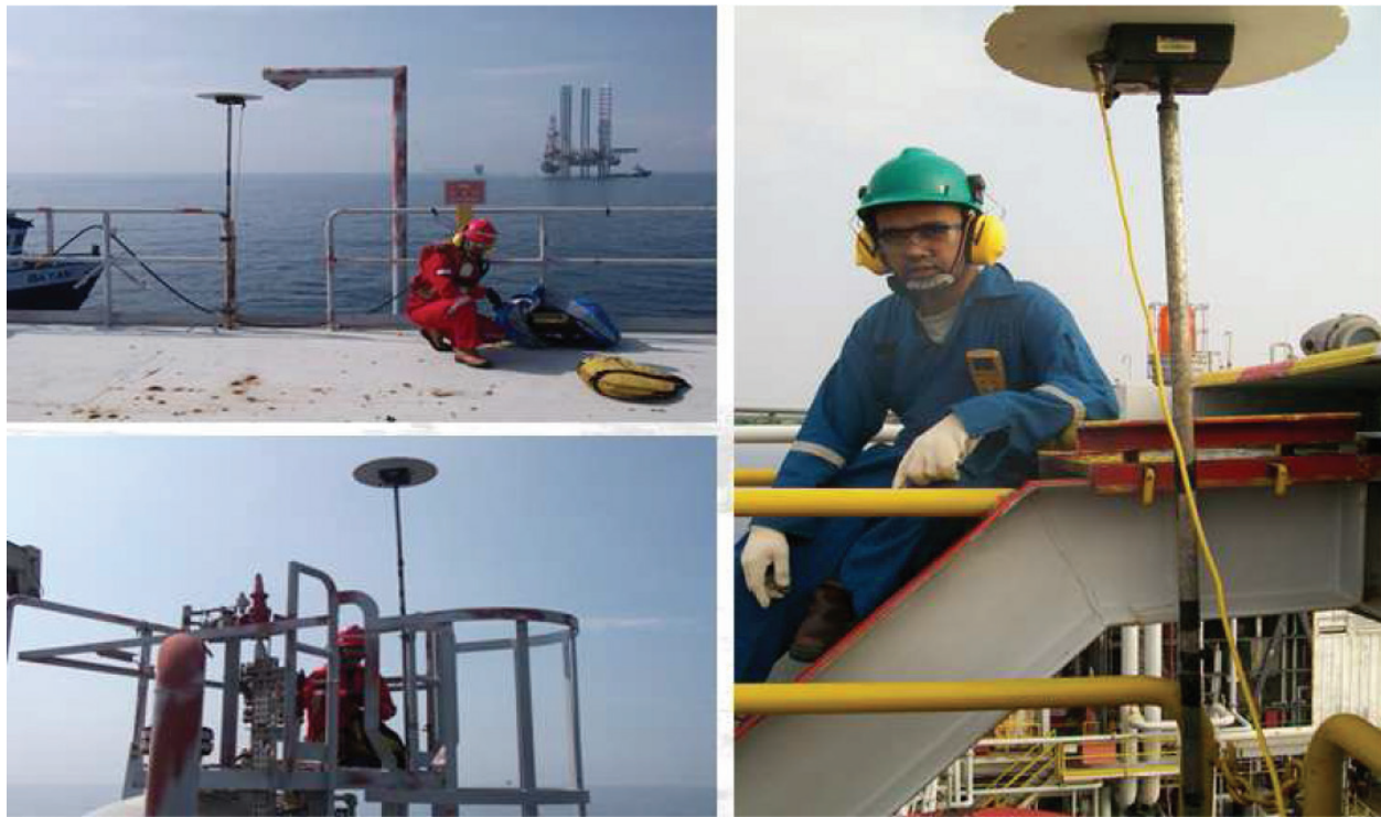
Figure 6. Illustration of GNSS GPS data acquisition in the field for oil and gas platform subsidence monitoring.
