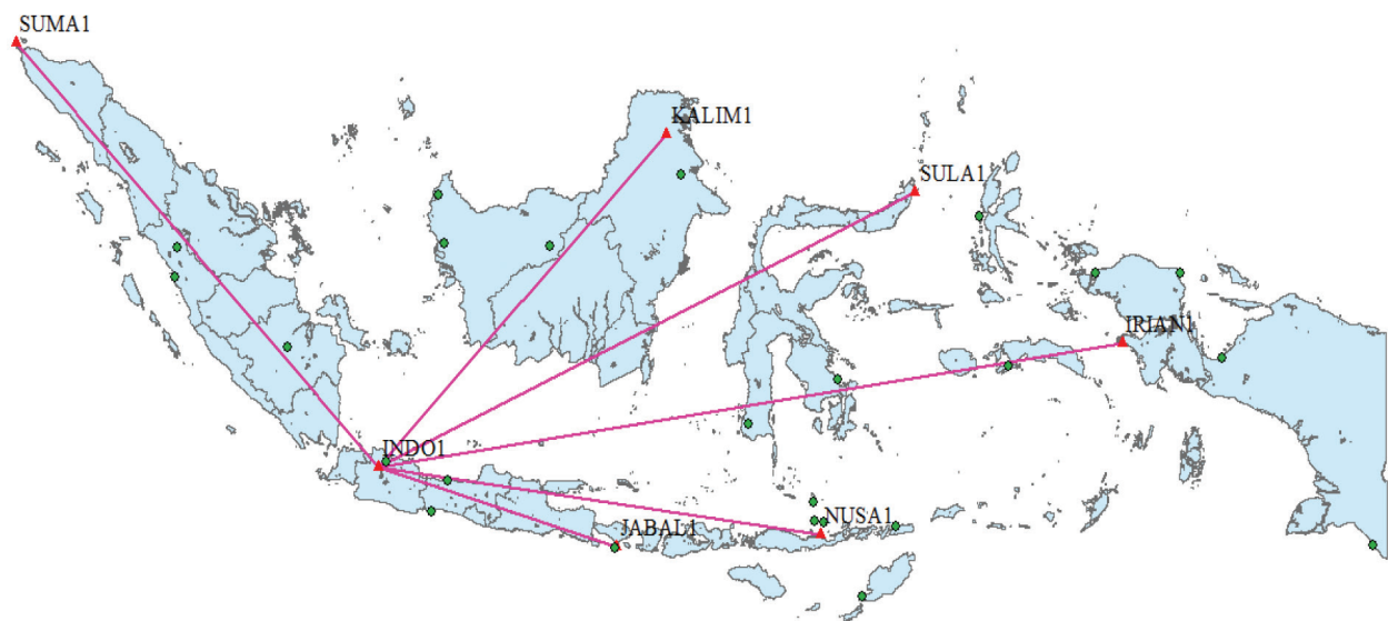
Figure 8. Baseline concepts using one stable reference station for subsidence monitoring along large offshore oil and gas area of Indonesia.
