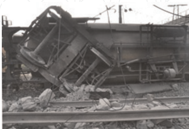
Figure 8. Plowing mechanism of the track by the bogie of the overturned carriage.
