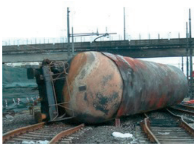
Figure 14. Front view of carriage no. 1 in the accident scene and position of its front bumper.
