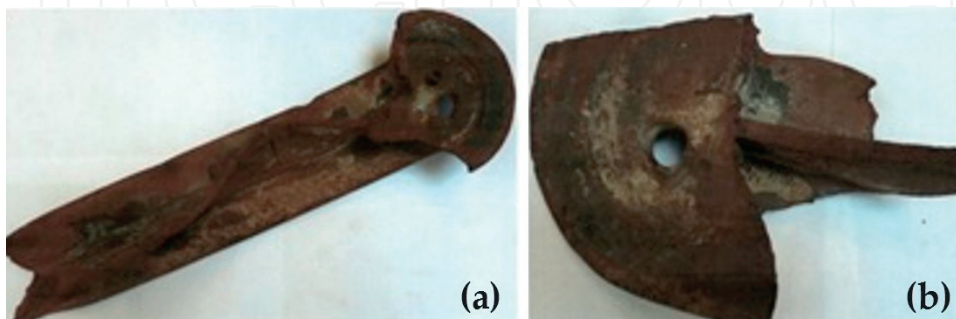
Figure 26. Two of the three chunks of the right axle box of the front wheel set of the front bogie of carriage no. 1: (a) chunk of the axle box found between the rails near the deformed check rail and (b) chunk of the axle box greatly abraded by the granite sidewalk curb exerting a grinding action on the right axle box, found externally to the track near the right-side rail in the train motion direction.
