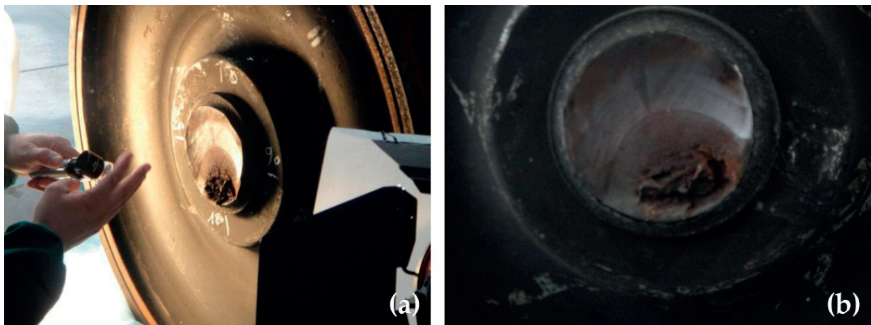
Figure 1. (a) Fatigue failure of the fracture surface of the axle on the wheel side. (b) Presence of a smooth area related to the slow propagation of the fatigue crack and of a rougher area of rapid failure of the residual axle section.
