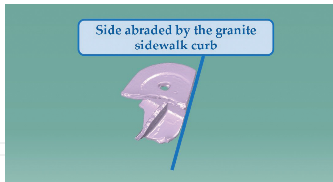
Figure 27. Digital twin of the chunk of the right axle box of the first wheel set of the front bogie of carriage no. 1 obtained by reverse engineering reconstruction based on geometry acquisition with a structured light optical sensor.
