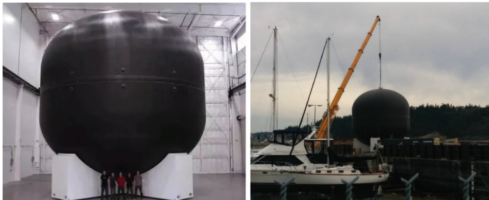
Figure 16. The 12-m diameter composite lox tank of space X.
