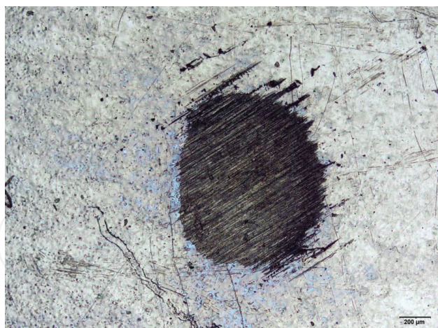
Figure 3. Wear test conducted on the ISO 5832-1 SS without laser treatment. Ball of AISI 316 L SS.
