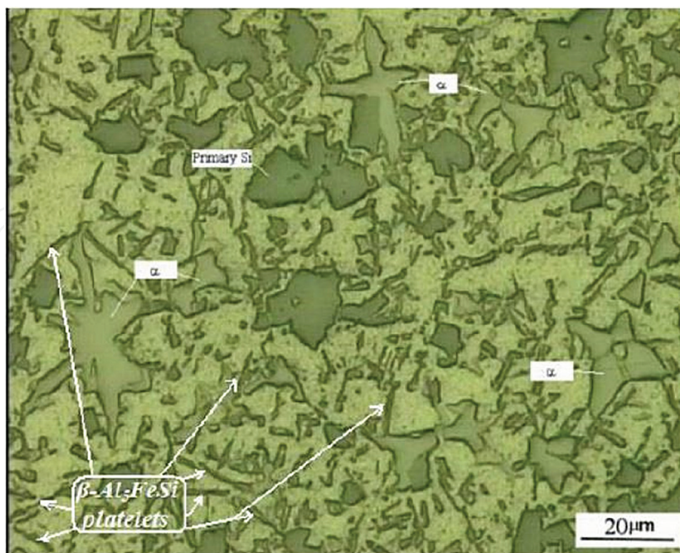
Figure 8. Optical micrograph of Al-Si-1.8Fe-0.8Mn microstructure [41].
