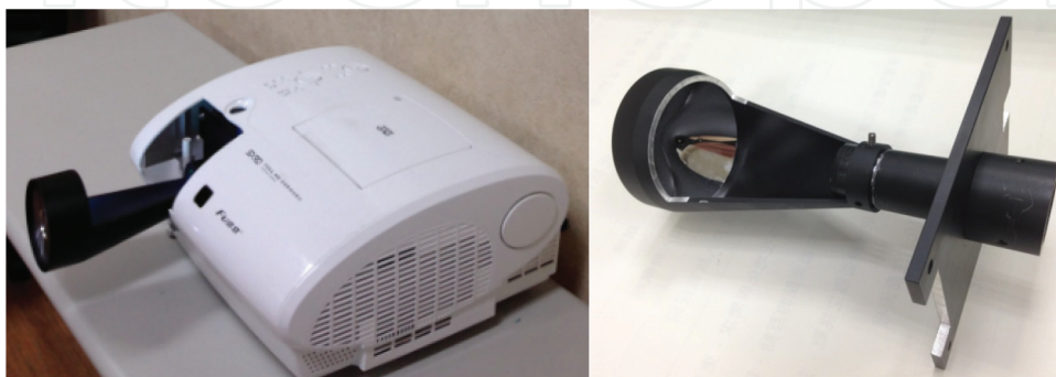
Figure 19. Utmost Co. LCoS projection engine with the self-designed optics and opto-mechatronic mount.
