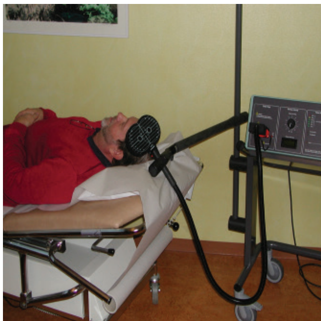
Figure 2. Position of a “patient” received TMS treatment with a figure-8 coil. The schematic drawing shows the induced electric field in tissue. Photo: Kjell Hansson Mild, drawing courtesy of Shoogo Ueno, Tokyo.
