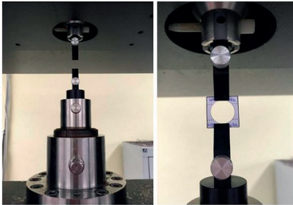
Figure 6. Single fiber disposition in the dynamometer MTS.
