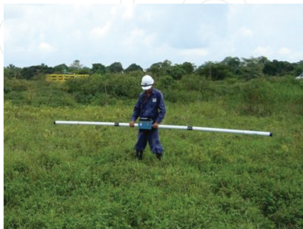
Figure 2. EM31-MK2 ground conductivity meter in field operations [12].
