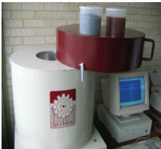
Figure 7. Low background scintillation detector NaI (TI), 325 Lab, D building, Faculty of Chemistry, UNAM.
