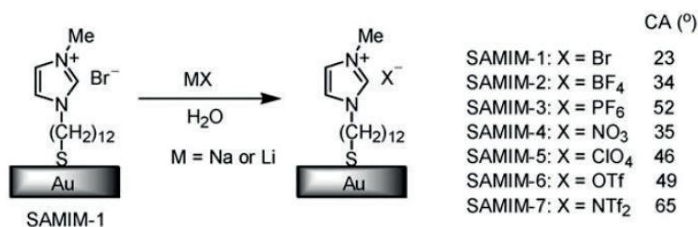
Figure 1. Grafting of monolayers on smooth gold substrates with imidazolium groups with sensitivity to ion exchange and surfaced hydrophobicity as a function of the ion-exchanged. Ref. [1], Copyright 2004. Reprinted with permission from American Chemical Society, USA.
