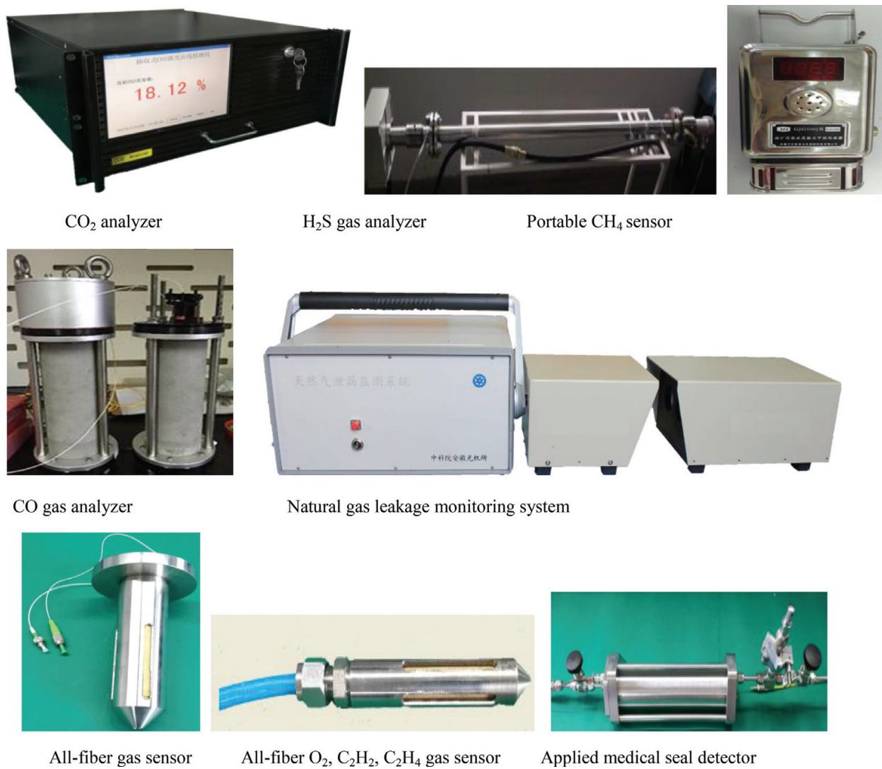
Figure 1. Several pictures of the TDLAS system developed by our research team.
