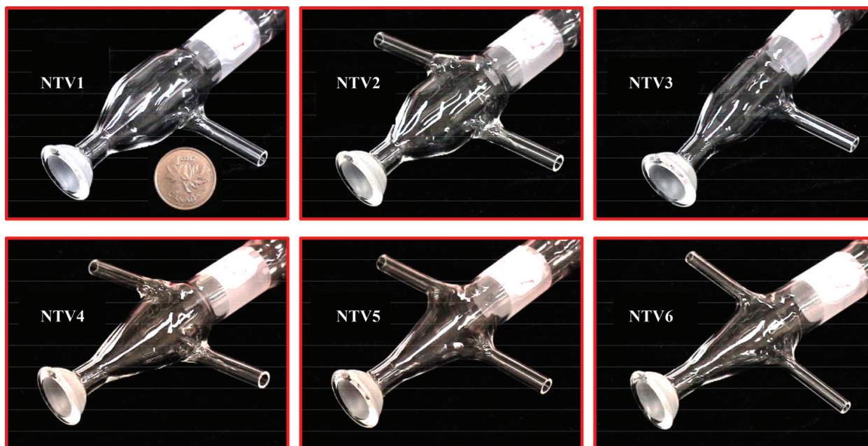
Figure 17. NTV vaporization chambers fabricated as a result of the CFD simulations. Dimensions listed in Table 2 . A Canadian penny (a 1 cent coin) has been included for size.
