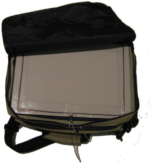
Figure 12. Dummy coil on the outer pocket of the bag
