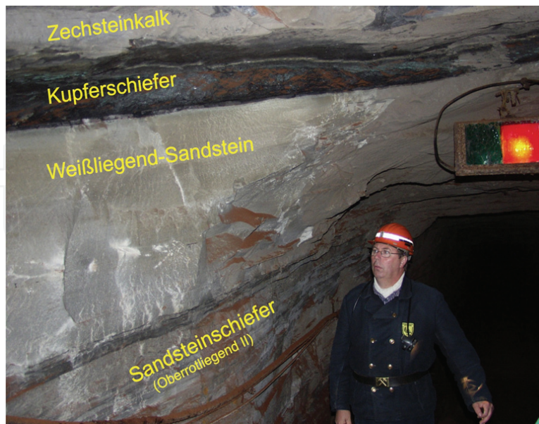
Figure 3. The upper Permian-lower Triassic sequence is from upper (Sandsteinschiefer) Rotliegend sandstone in the footwall, the mineralized Weißliegend white sandstone and Kupferschiefer metallized black shale, and the hanging wall of Zechstein dolostone. Location: Roerigschacht, Wettelrode/Sangerhausen mine, Mansfeld district, Germany. The Permo-Triassic boundary is placed at the Kupferschiefer-Zechstein contact. (Photo by Juergen Kopp showing the mine manager Dipl.-Ing. Erich Hartung).
