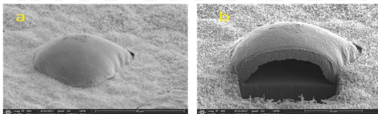
Figure 7. (a) SEM image of a Ga cluster on the surface of n-type GaAs oxidized at 942°C, (b) Closeup of the same cluster after etching with a focused ion beam, showing nanowires surrounding the cluster but none on top of it.
