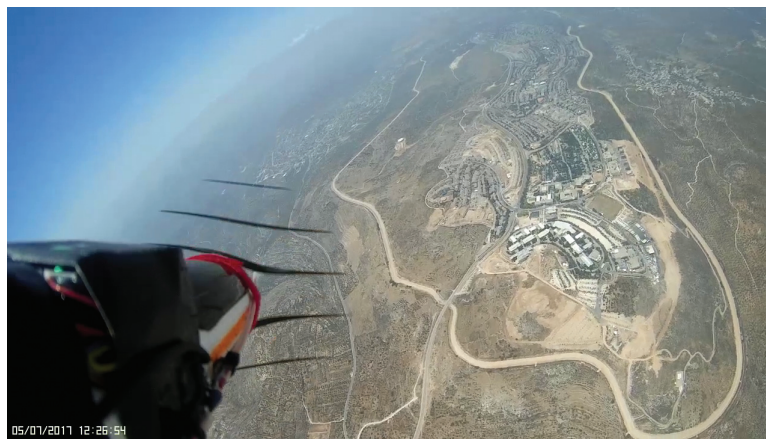
Figure 18. Getting back home: A massive UHF transition caused the drone to get into the “fail-safe” state, releasing the drone which in turn flew back to “home” autonomously.
