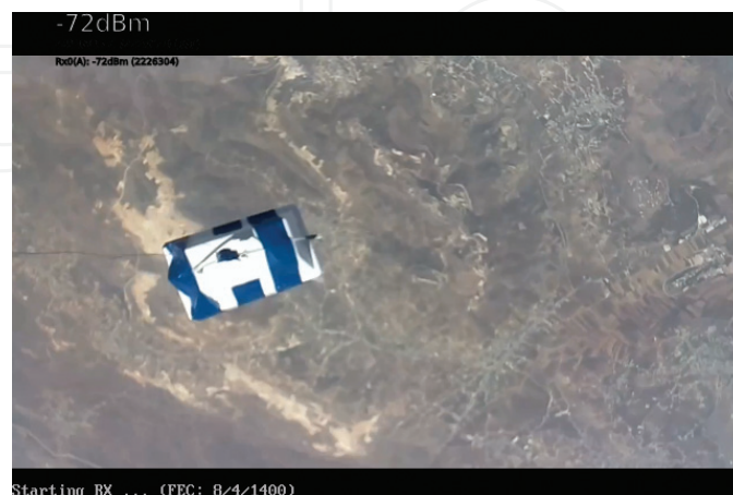
Figure 13. The smartphone payload shot from an upper payload based on a Raspberry-Pi camera equipped with a long-range Wi-Fi transmitter. The picture was taken at about 9.7 km above ground.
