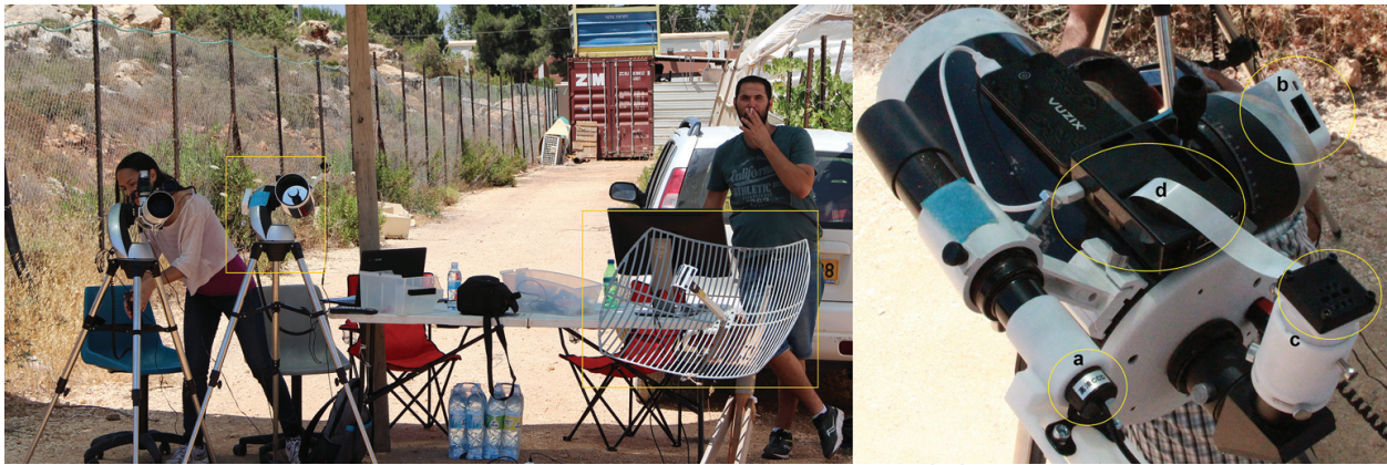
Figure 11. HAB ground station (GS): Left: The GS in general: two robotic telescopes with (auto-track) and a high gain 24dBi Wi-Fi antenna. Right: the robotic telescope: (a) A view-finder webcam. (b) A Wi-Fi + 3G router. So the telescope can be controlled globally. (c) A Pi-camera mounted to the telescope eye-view. (d) A Raspberry Pi which controls the telescope using either visual tracking and GPS coordinates.
