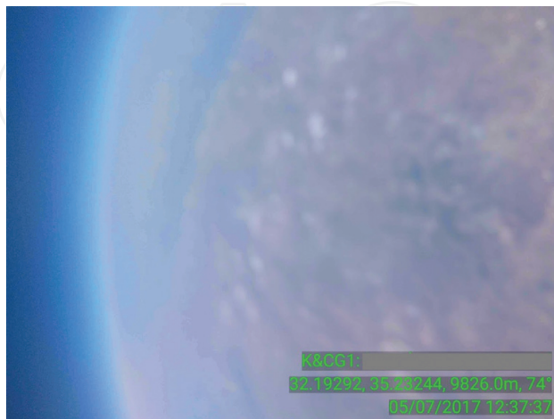
Figure 10. An image of the sky that was made by an android smartphone (Xiaomi Redmi 4A). In this experiment, the phone's camera was out of focus. It might be due to ice on the camera lens. The images were successfully uploaded after the payload has made it to the ground.
