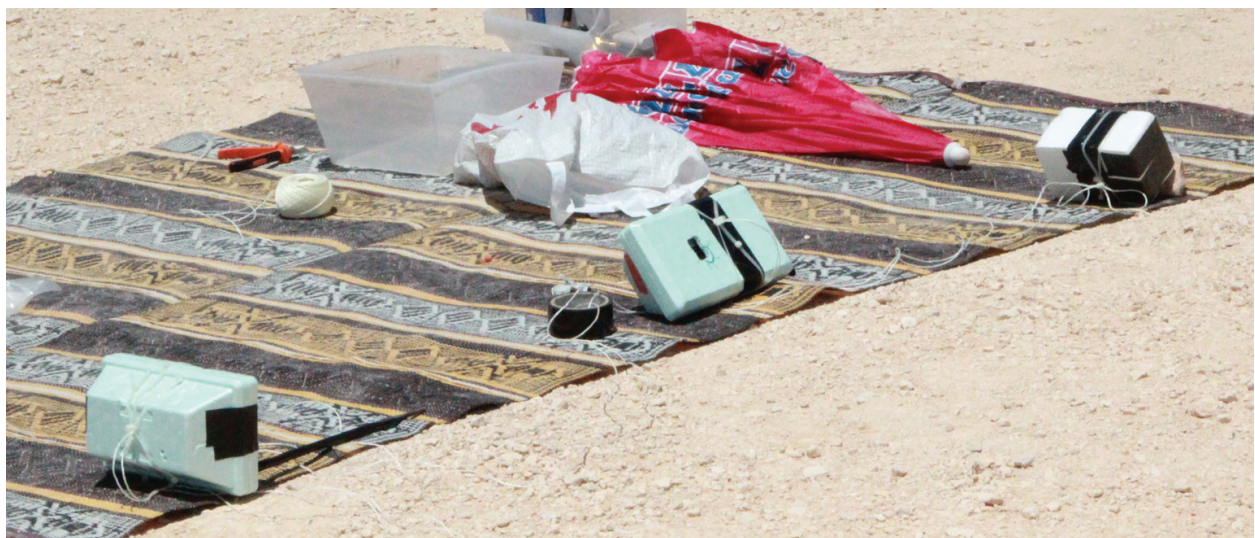
Figure 9. Three payloads ready to be launched—each with a smartphone and software for uploading the gathered data. As part of the navigation graduated course in Ariel University (Israel). None of the payloads could actually transmit good and clear images from high altitude. All payloads eventually fall in Suraya. Over 200 km from launch.
