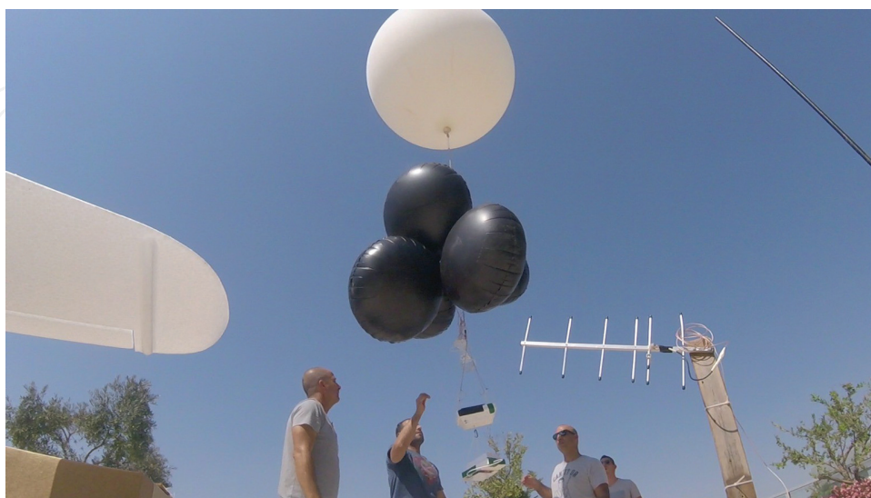
Figure 3. A long-lasting HAB experiment. This setting retained its floating state for about 2.5 h before the main balloon exploded.
