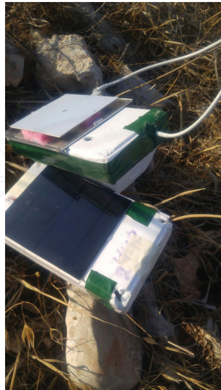
Figure 4. The retrieved payloads from the above experiment were found on a distant field, about 100 km from the point of launch. The crashing location was transmitted by the iridium communication system after the crash. In the picture, the upper box is the secondary payload and the main is the lower box.
