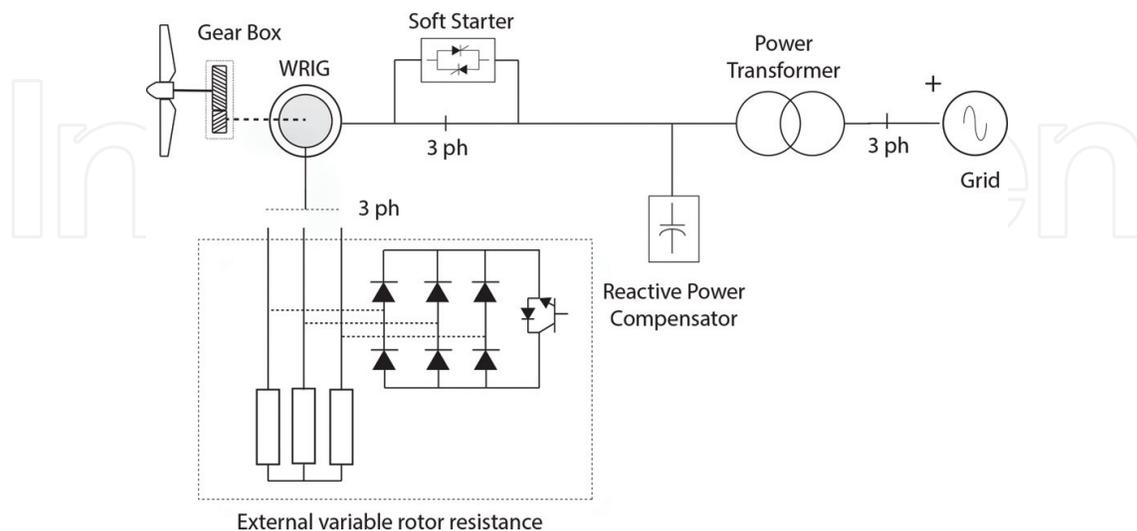
**Figure 4.** WRIG with external variable resistance configuration.
