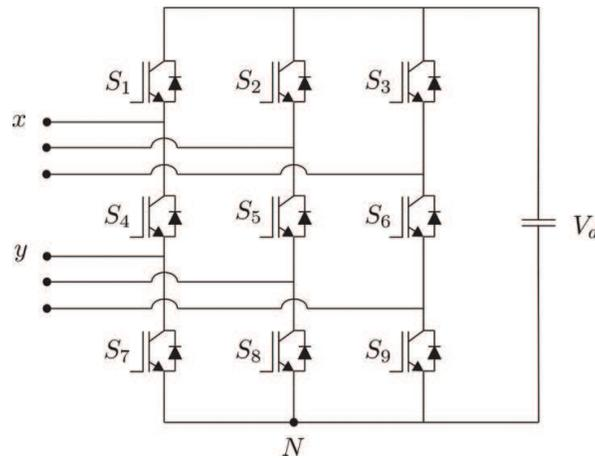
Figure 18. Nine-switch converter topology, rectifying stage.
