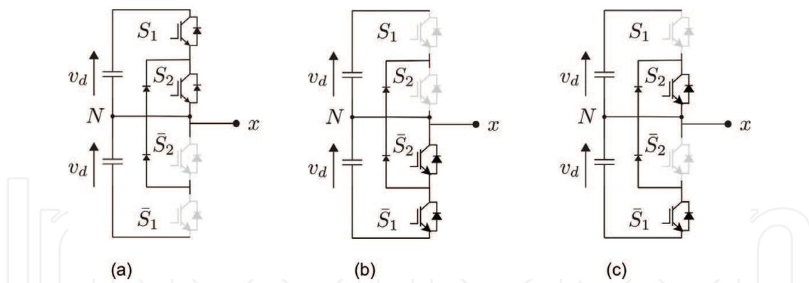
**Figure 12.** NPC LS-PWM switching states: (a) P state, (b) N state and (c) zero state.
