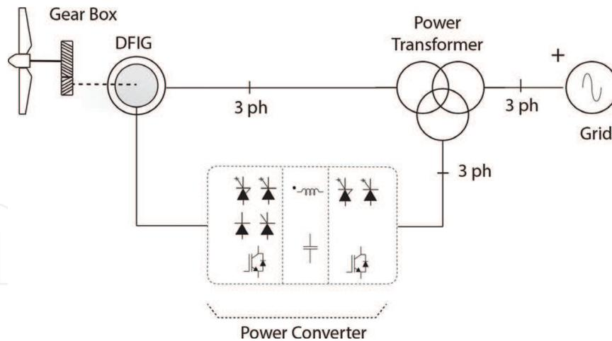
**Figure 5.** DFIG with partially rated power electronics configuration.
