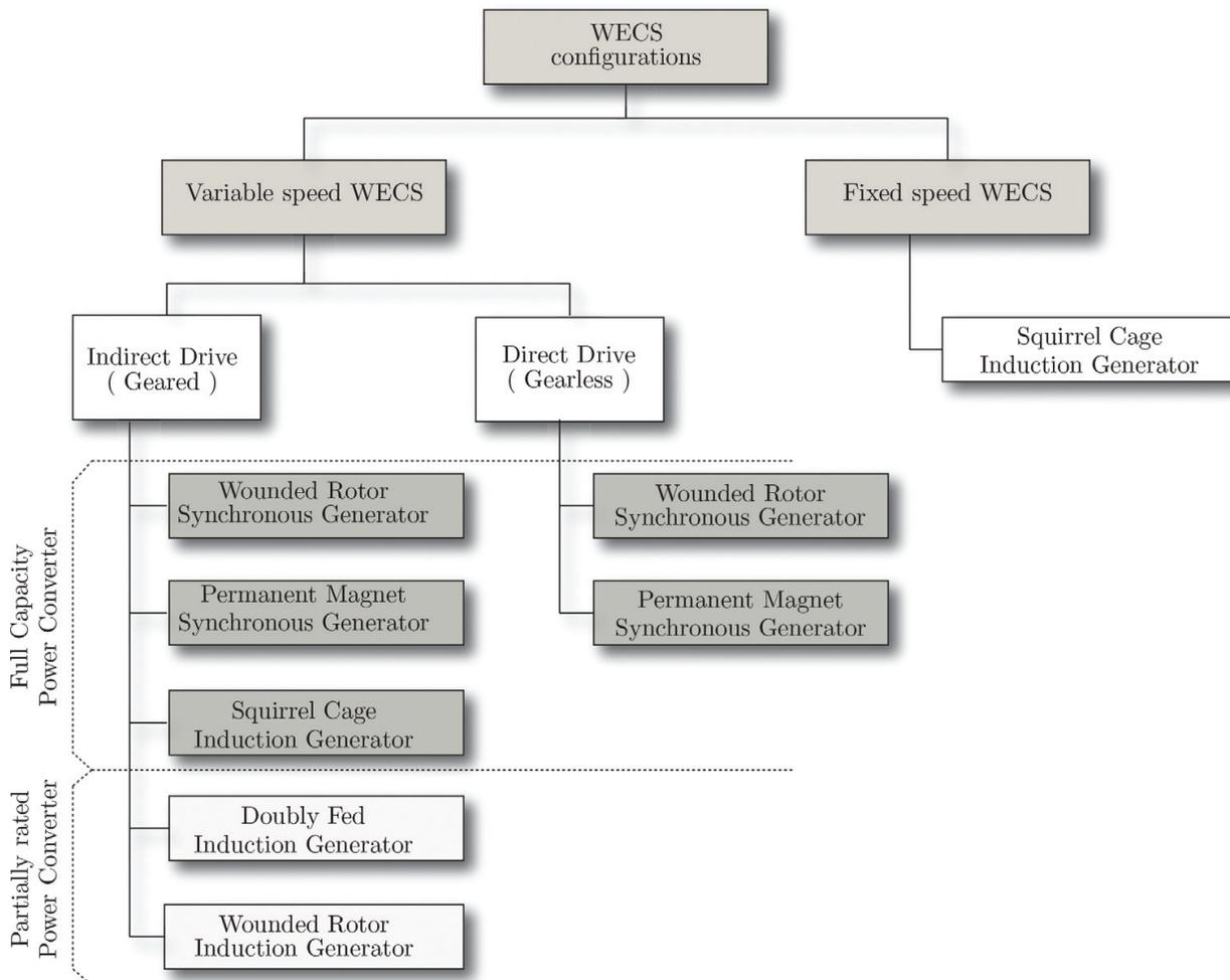
**Figure 2.** WECS configurations.
