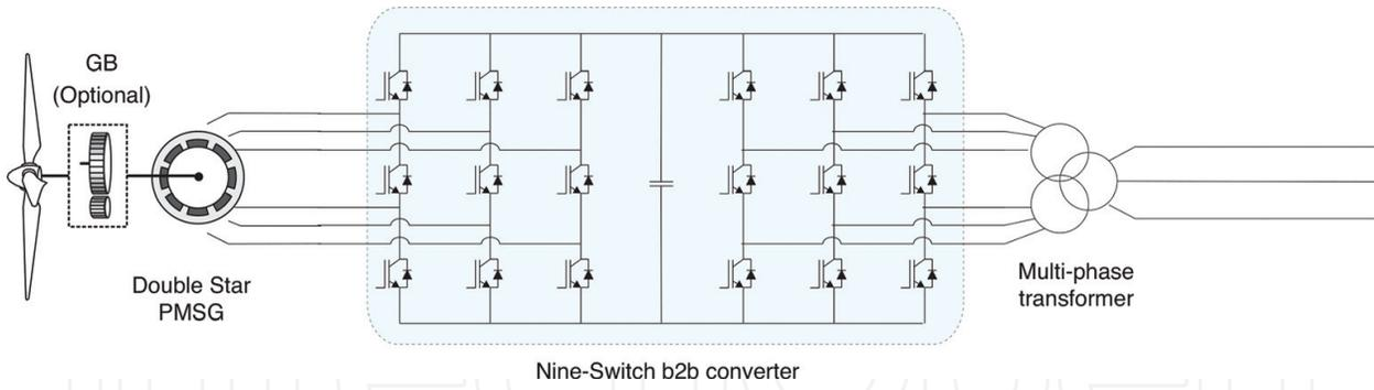
Figure 17. Nine-switch converter back-to-back topology.
